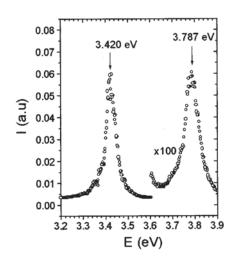
FIG. 5. Photoluminescence spectrum of an AlGaN/GaN structure (sample No. 5 in Table I). The peak positions in the photoluminescence spectrum were taken as band-gap energies of the AlGaN and GaN layers, respectively, as indicated by arrows.
