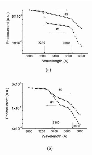
FIG. 4. Normalized photocurrent as a function of the wavelength of the incident light of an AlGaN/GaN heterostructure. (a) for sample No. 9 and (b) for sample No. 5 in Table I. Curve 1 was obtained by scanning from low photon energy to high photon energy and curve 2 was obtained in the reverse direction, the horizontal arrows indicate the direction of scanning in wavelength. The vertical arrows indicate the band-gap wavelength of GaN and AlGaN.
