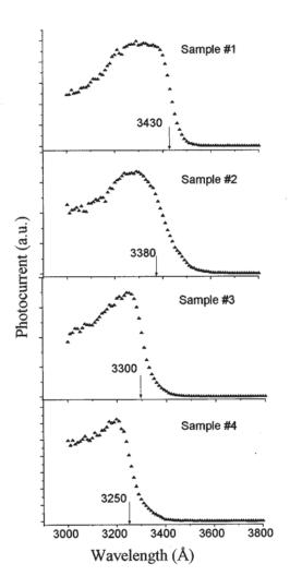
FIG. 3. Normalized photocurrent of bulk AlGaN samples as a function of the wavelength of the incident light. The arrows indicate the wavelength responding to the band-gap energy of AlGaN obtained by the maximum slope of  $dI/d\lambda$ . The results are listed in Table I.
